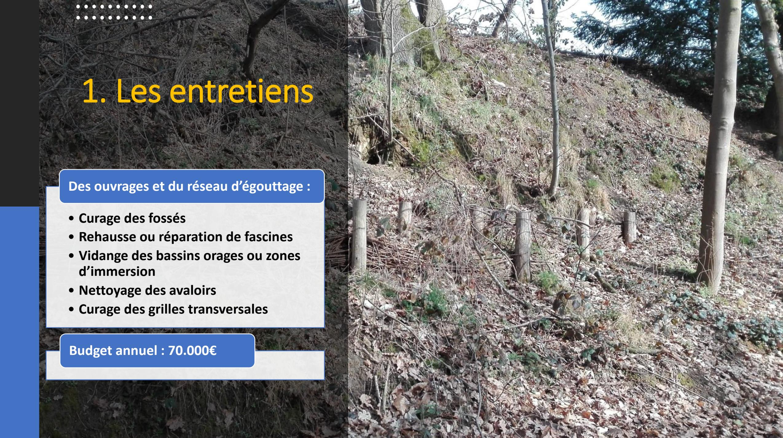
The background image shows a steep, wooded slope covered in dry leaves and twigs. A series of vertical wooden posts are driven into the ground, connected by a horizontal layer of brushwood (fascine) to form a drainage structure. The trees are mostly bare, suggesting an autumn or winter setting.
